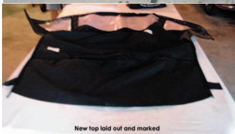
New top laid out and marked
